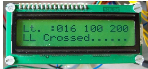
Figure 2: Lower limit crossed; hence the relay in figure 1 switches OFF.
