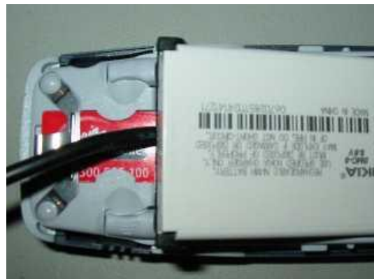
Figure 4-4.1b F-bus connected to 3310
