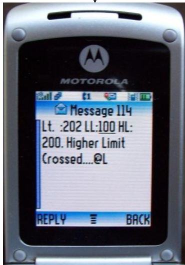
Figure 3 Warning received on mobile as higher limit crossed
